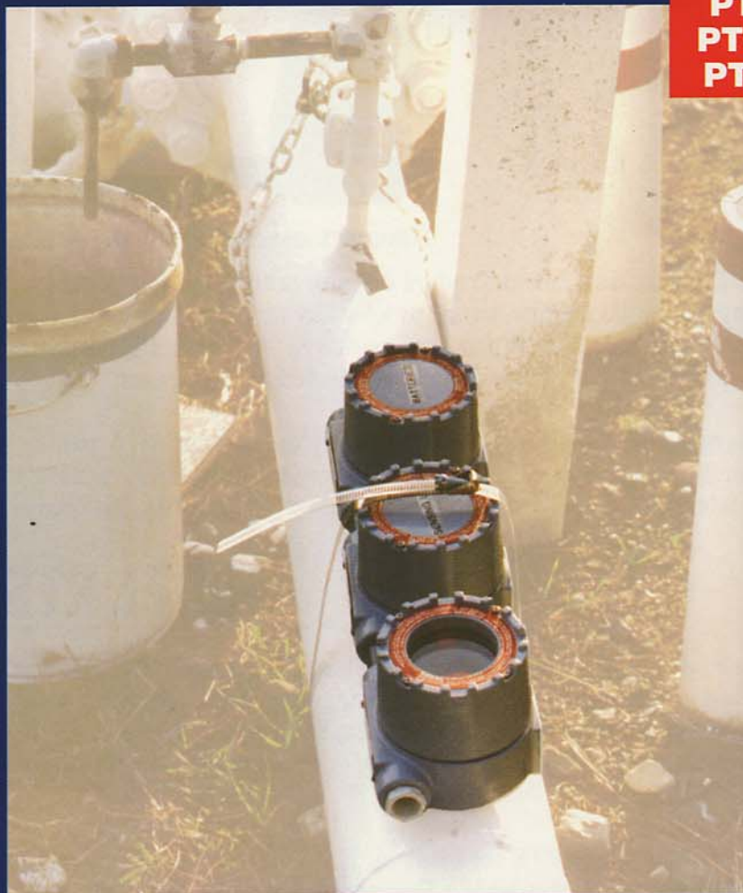
Model PTS strapped in place on pipe. In this application, the sensor signalled the launching of a series of pigs. The Model PTS was then moved to the end of the run to signal the arrival of each pig.
