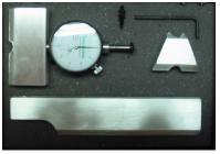
Vessels, and other complex curvatures, such as pump housings, valve bodies, impellers, turbine blades, etc. As the name suggests, the Pocket Pit Gauge conveniently fits in your pocket (but then again so does the Basic Pit Gauge).
